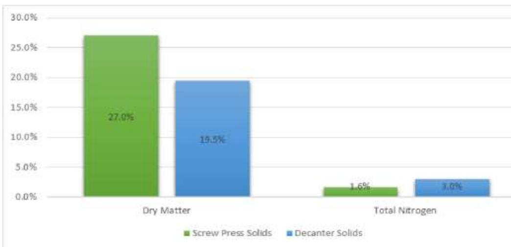
Figure 2. Comparison between solids obtained from the screw press and decanter centrifuge. Separately, screw press solids are much higher in DM content albeit lower in N, possibly indicating that a substantial proportion of inorganic nitrogen is dissolved (and, therefore, chemical separation is needed). Nutrient analysis undertaken and verified by NRM laboratories.
