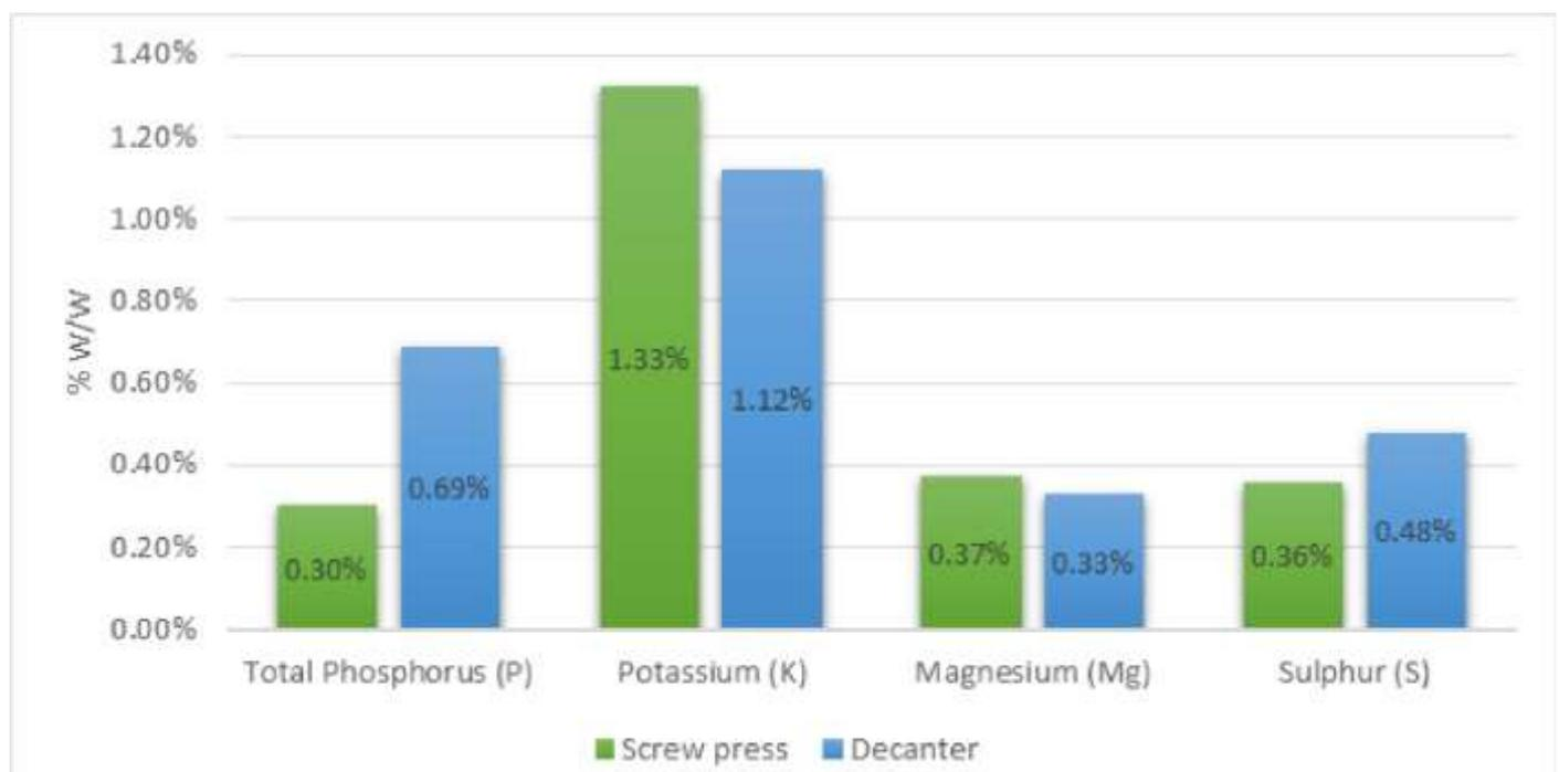
Figure 3. Comparison between several nutrient concentrations within the screw press and decanter centrifuge solids. The screw press is shown to obtain the bulk of these nutrients, nevertheless, the decanter (with chemical amendment) is more effective at removing P and S considering there is a lower concentration of these in the
