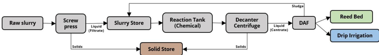
Figure 1. Flow diagram of the dewatering process. Until December 2021, filtrate was placed in the slurry store and was diluted with yard/parlour washings, however filtrate now remains undiluted by entering the reaction tank straight after the screw press separator – this represents both ways in which slurry/washing can be stored on farm (separately and together).
